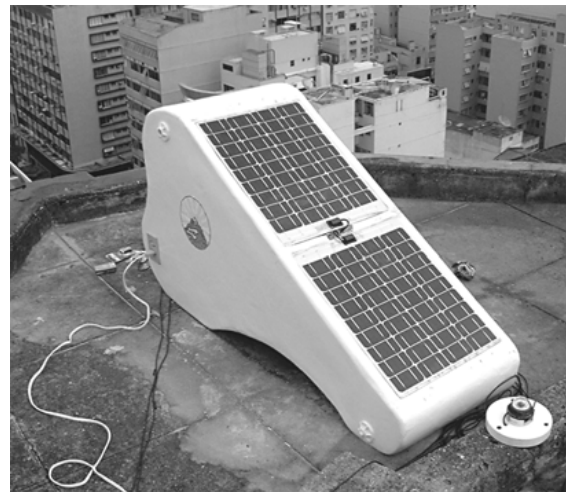
Figure 6: The first I-SHS prototype during tests in Copacabana, Rio de Janeiro, Brazil in 2002. Design by “Escola de Belas Artes”, UFRJ, Rio de Janeiro (modified by Fabian Ochs).
