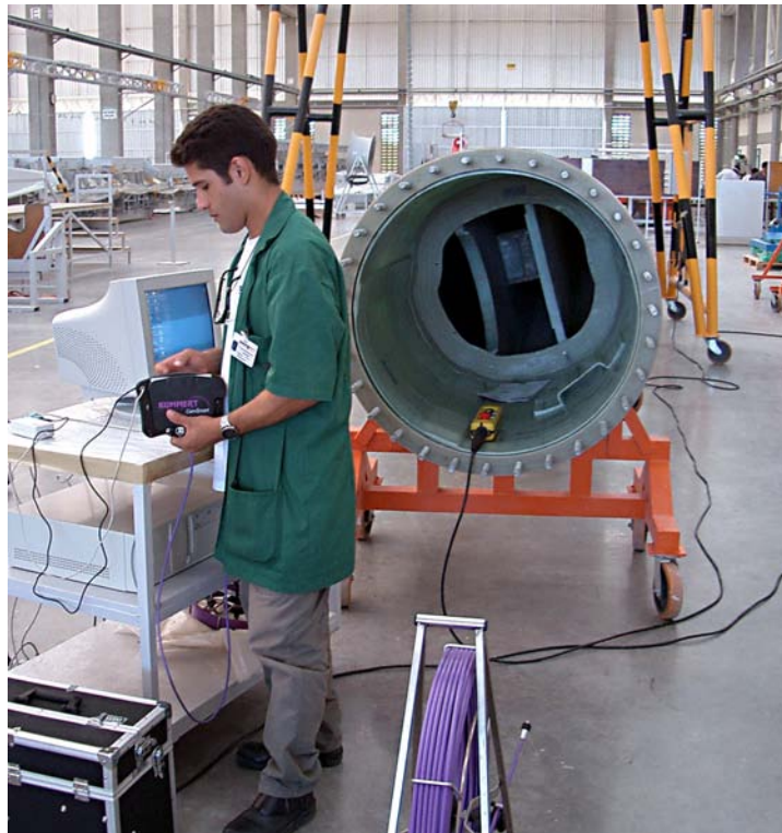
Figure 3: Final check via an online-endoscope inside a blade for a 600 kW wind turbine at Wobben-Enercon in Pecém (35 km west of Fortaleza): Still Latin America's only manufacturer for large scale wind turbines.
