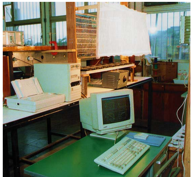
Fig.1. PV-Facade with cooling and cloud-filter for investigations on thermal and optical performance and parameters.
