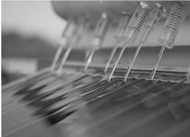
Fig. 1. Creation of the water film on the PV module by a line of nozzles.
