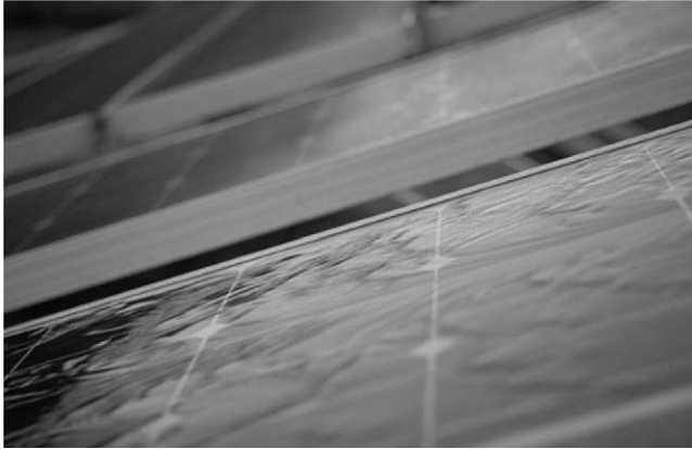
Fig. 5. Close-up of the flowing film of water at the PV module surface.
