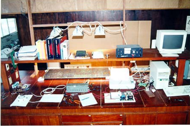
Fig.2. Charging device with PV-module and solar simulator at Laboratorio Fotovoltaico at UFRJ-COPPE/EE.
