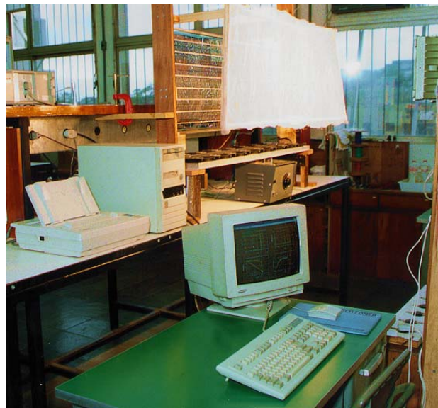
Fig.1. PV-Facade with cooling and cloud-filter for investigations on thermal and optical performance and parameters.
