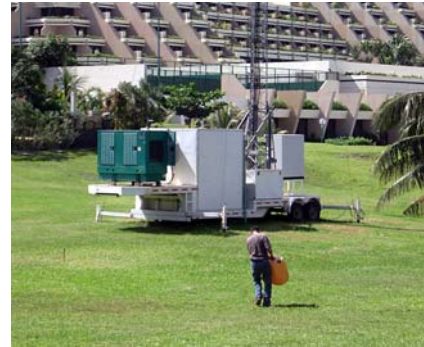
Figure 6: Diesel-powered cellular phone transmitter with refilling-boy arriving (Cancun, Mexico): noise, smoke, frequent fuel refills – why not PV?
